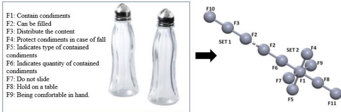
Figure 5 A salt cellar and its 3D modular graphical representation. Adapted from Boyard et al. (2015).
