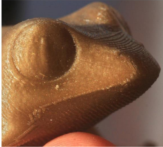
Figure 20 Stair-case effect on a 3D printed frog (Francois, 2013).
